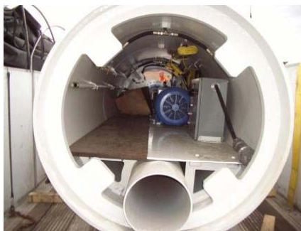
The 'Inner Works' of a Tunnel Boring Machine' (TBM)
